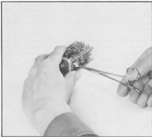
Fig. 4-2. Removal or replacement of sampling bridge diodes.
